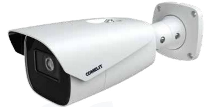
**LA CAMÉRA IPLPRA04ZSWA MARQUE UNE AVANCÉE SIGNIFICATIVE DANS LES SYSTÈMES DE LECTURE DE PLAQUES D'IMMATRICULATION, EN INTÉGRANT LA NORME WIEGAND W26 POUR PERMETTRE L'INTERFAÇAGE AVEC LES SYSTÈMES DE CONTRÔLE D'ACCÈS.**
